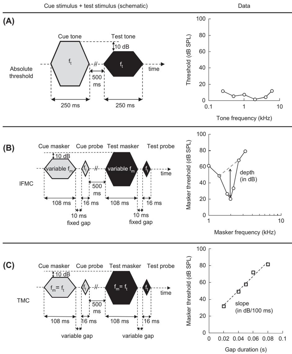
**Figure 1.** First column: schematic representation of the test stimuli in measures of (A) absolute threshold (250-ms tone), (B) iso-forward masking contour (IFMC), and (C) temporal masking curve (TMC) measure. Second column: examples of the data obtained in the absolute threshold, IFMC (with  $f_t = 2$  kHz) and TMC measure for a listener with good hearing, plus illustration of depth and slope measure for IFMC and TMC respectively.
